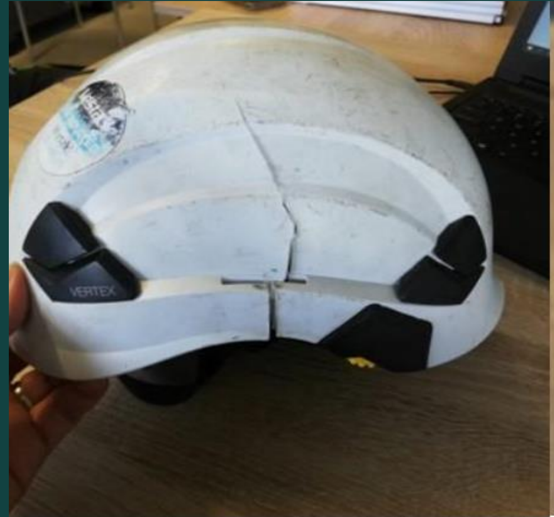
Fig 7. – cracked and dented (marked) IP's hard hat
