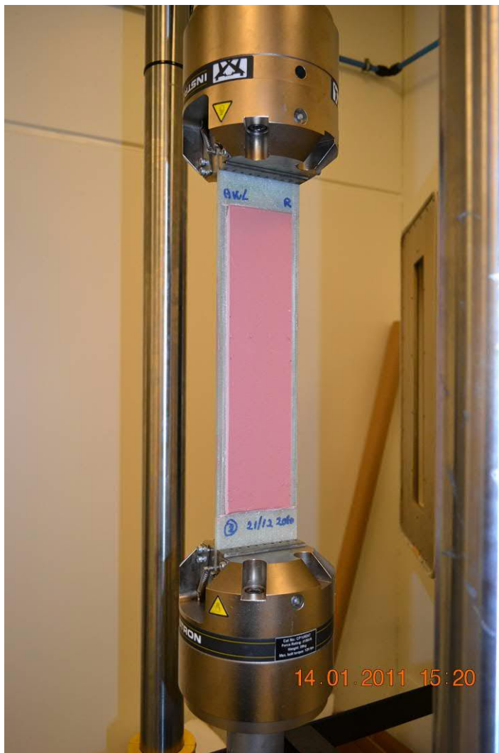
Figure 9. Example of specimen with filler only ready for fatigue testing.
