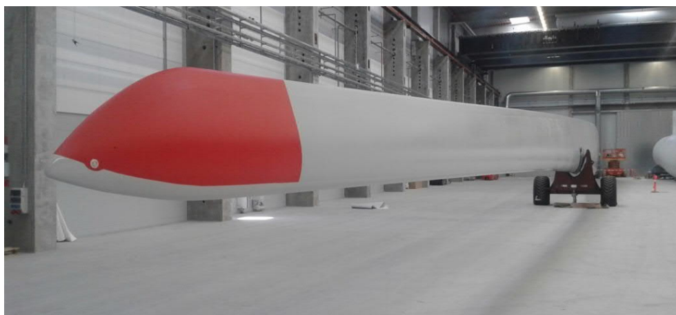
Figure 3. Liquid LEP applied to an SGRE blade.
